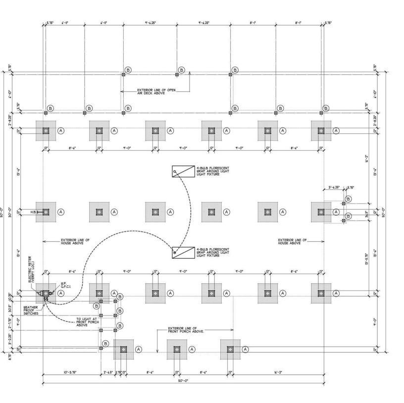
FOOTING: 42\*X42\*X2\* CONC. FOOTING W/4-NO. 5 RE-BARS AT 4\* 0.C. EACH WAY AND 4\* FROM EDGE. COLUMN: 12\*X12\*X8\* CONCRETE COLUMN BLOCK COLUMN W/4-NO. 5 REBARS VERTICAL (GROUT SOLID)
