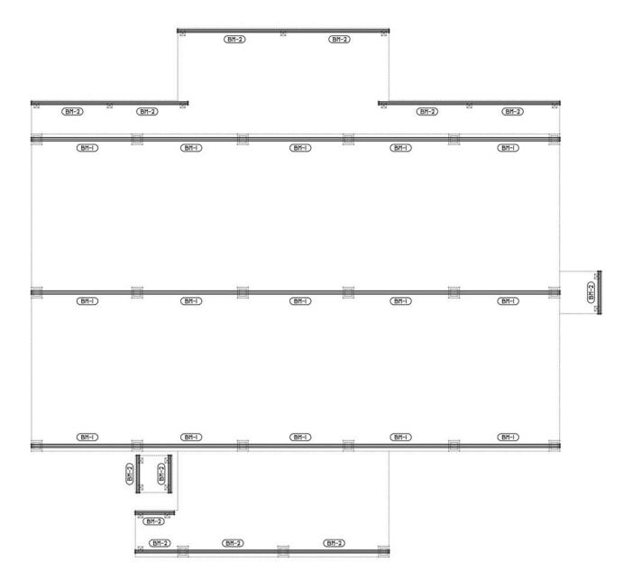
(BM-I) = (2) 1.75" X 11.25" 2.0E GP LAM (BM-2) = (2) 2"X12" P.T. WOOD BEAM
